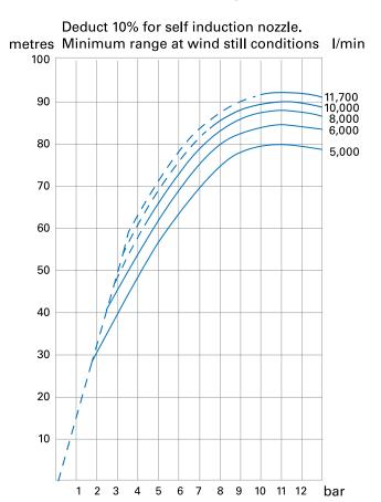
Reaction force (N) =  $0.233 \times Q$  (I/min)  $\times \sqrt{p}$  (bar)
