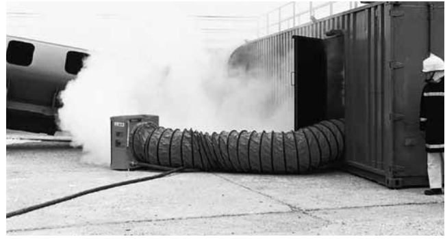
Fomax 7 as smoke extractor (smoke extractor model)
